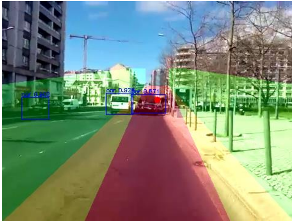
Figure 3.1.1 – Risk assessment framework: The estimation of the Focus of Expansion (red point) allows a representation of different level risk areas in the image. Risk is evaluated taking into account the objects in the image (blue rectangles) and the path of the cyclist (red area in the image).
