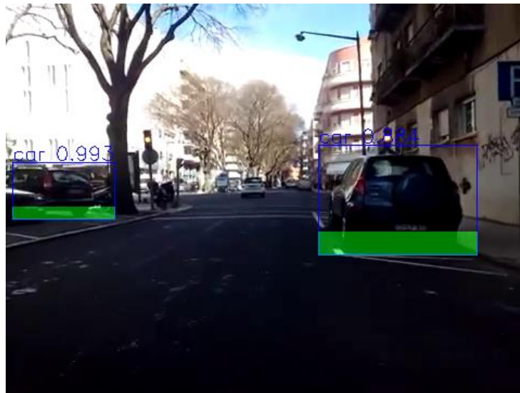
Figure 4.2.3 – Boxes of the objects. In blue, the bounding box given by the NN is shown, whereas in green it is shown the box of the alternative box used as a projection of the object on the ground.
