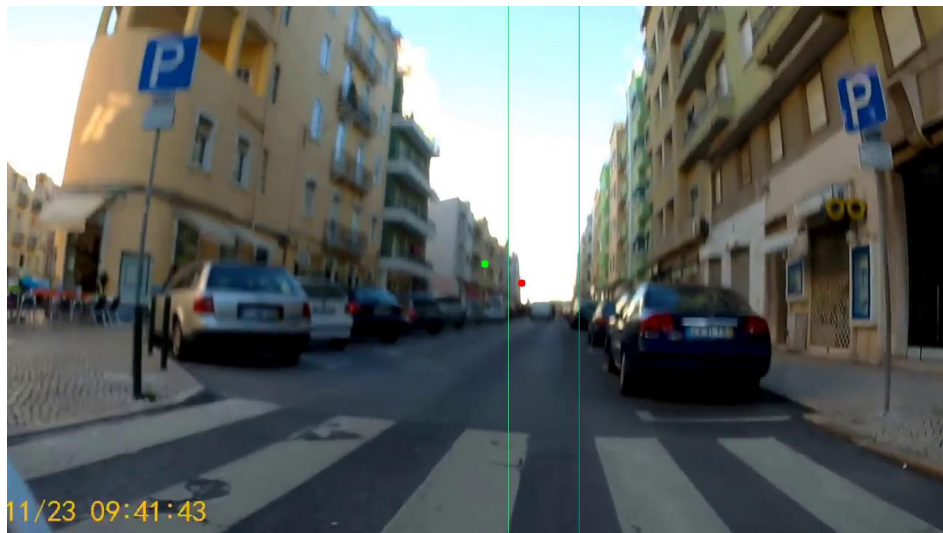
Figure 4.3.2 - Turn Right event. It is shown the current FOE (red point), the previously averaged FOEs (green point) and the thresholds for the Smooth Turn Right (green line) and for the Sharp Turn Right (cyan line). It is seen, that because the red point is to the right of the green line, there is currently a Smooth Turn Right movement.
