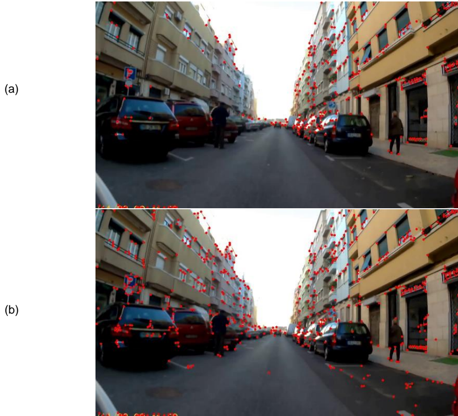
Figure 4.1.2 - Features tracked using the Shi-Tomasi method [37] in red. In (a) the features are calculated on the whole image and in (b) features are calculated using the image separation into 16 sub-images.
