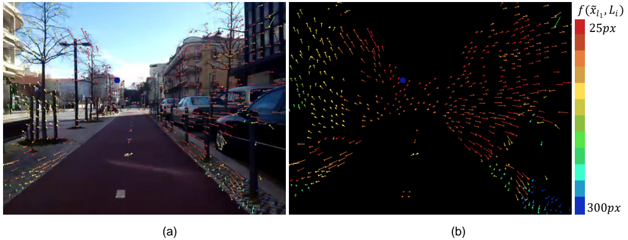
Figure 4.1.5 – Heatmap of the distance between lines L_i and the estimation of the FOE given by the Huber Loss Distance optimization calculation.
