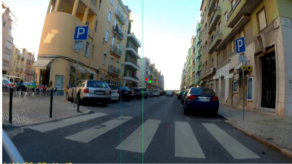
Figure 4.3.1 – Turn Left event. It is shown the current FOE (red point), the previously averaged FOEs (green point) and the thresholds for the Smooth Turn Left (green line) and for the Sharp Turn Left (cyan line).
