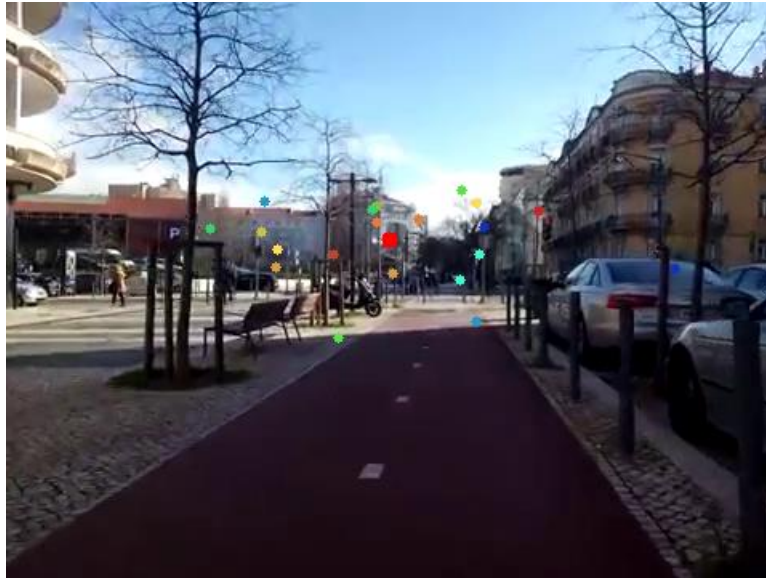
Figure 3.6.1 – The weighted average of the previous and current FOE (small coloured points) and the result of this operation (large red point in the centre of the image).
